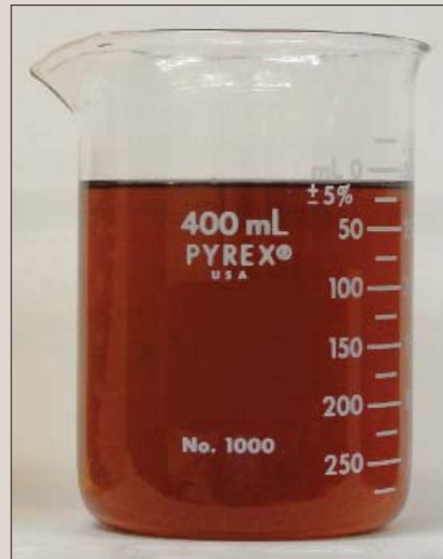
Same samples after 1,300 hours of exposure @ 200°F
