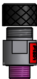
Model of valve stem 5/8" 18 UNF 1A (A)
