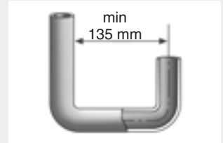
● Minimum clearance of U-shape bends
