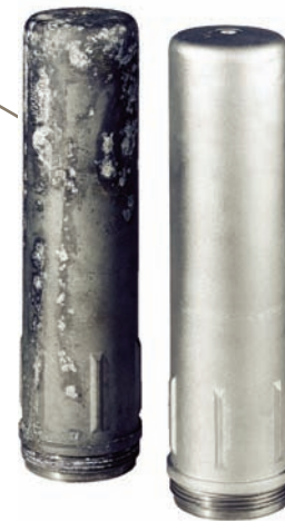
Untreated and Alu-chromed filter bowls after a salt spray test acc. to DIN 50021 SS > 250 hours
