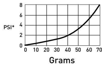
Racor Gasoline Solid Capacity Test (using SOFTC-2A; 10 mic. Element)
