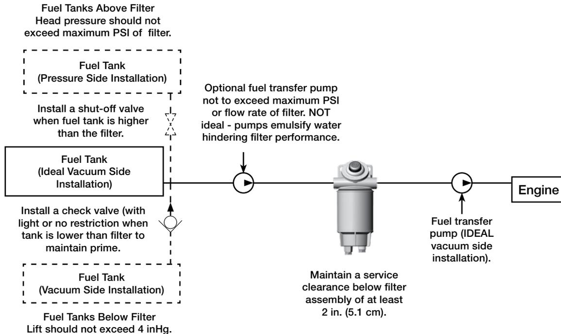
Installation diagram applies to all 400 Series filters. Model 445MAM10 shown above. Racor offers hose and fittings to complete this installation. See Marine Accessories.
