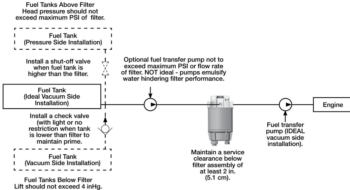
Installation diagram applies to all 200 Series filters. Model 215RMAM shown above. Racor offers hose and fittings to complete this installation. See Marine Accessories.
