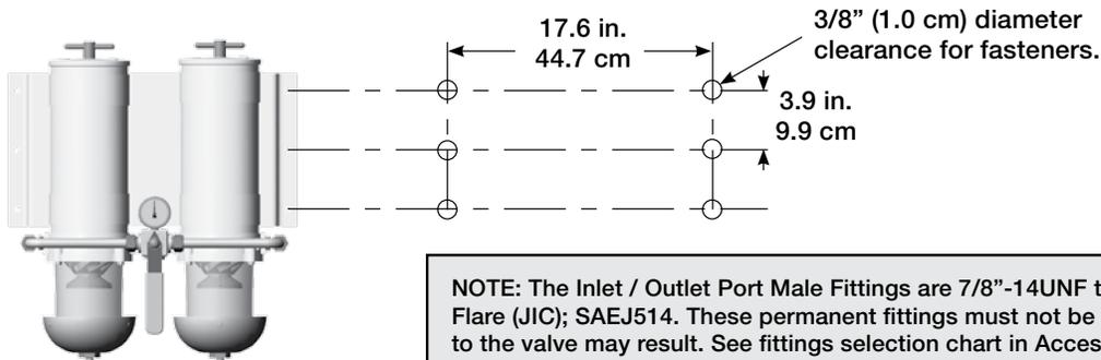
NOTE: The Inlet / Outlet Port Male Fittings are 7/8"-14UNF threads with 37° Flare (JIC); SAEJ514. These permanent fittings must not be removed. Damage to the valve may result. See fittings selection chart in Accessories Section to adapt to your fuel system piping requirements.
