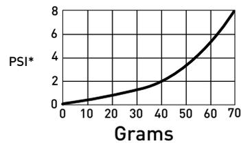
Racor Gasoline Solid Capacity Test (using SOFTC-2A; 10 mic. Element)
