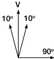
Note: 1. Mount filter assembly as close to vertical (V) as possible. For best efficiency, do not exceed 10° from V.
